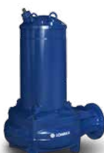
Lowara 1335 Non-clog Maximum flow 492 l/s Maximum pressure 55 m Motor Rating 18 - 50 kW Outlet 150 - 300 mm Weight 580 - 760 kg
