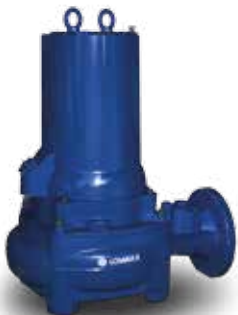
Lowara 1325 Non-clog Maximum flow 115 l/s Maximum pressure 63 m Motor Rating 9 - 18 kW Outlet 80 - 150 mm Weight 170 - 190 kg
