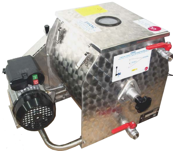
① Unit: EMANC. Computer Controlled Butter Maker Teaching Unit
