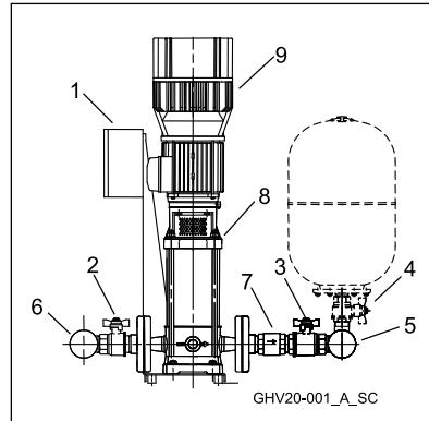
The check valve may be located on the delivery or suction side, depending on the type of set; the electric pump may be vertical or horizontal type. The tank is not included in the supply.
